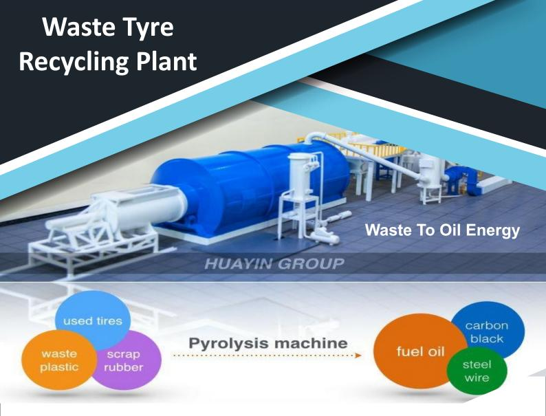
Pyrolysis is the chemical decomposition of organic materials by heating in the absence of oxygen or any other reagents, except possibly steam.
