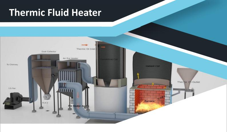
"Thermic Fluid Heaters are heating equipment, used in industry where heat transfers are primary need of process instead of pressure."
