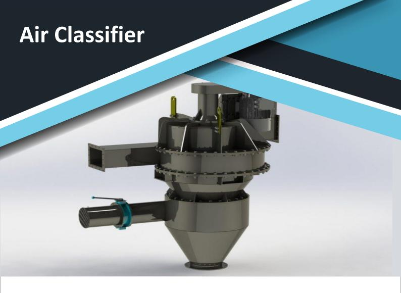
An air classifier is an industrial machine which separates materials by a combination of size, shape, and density. It works by injecting the material stream to be sorted into a chamber which contains a column of rising air.
